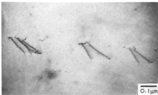
Figure 8 Electron micrographs of slightly abraded (1 0 0) GaP specimen.
